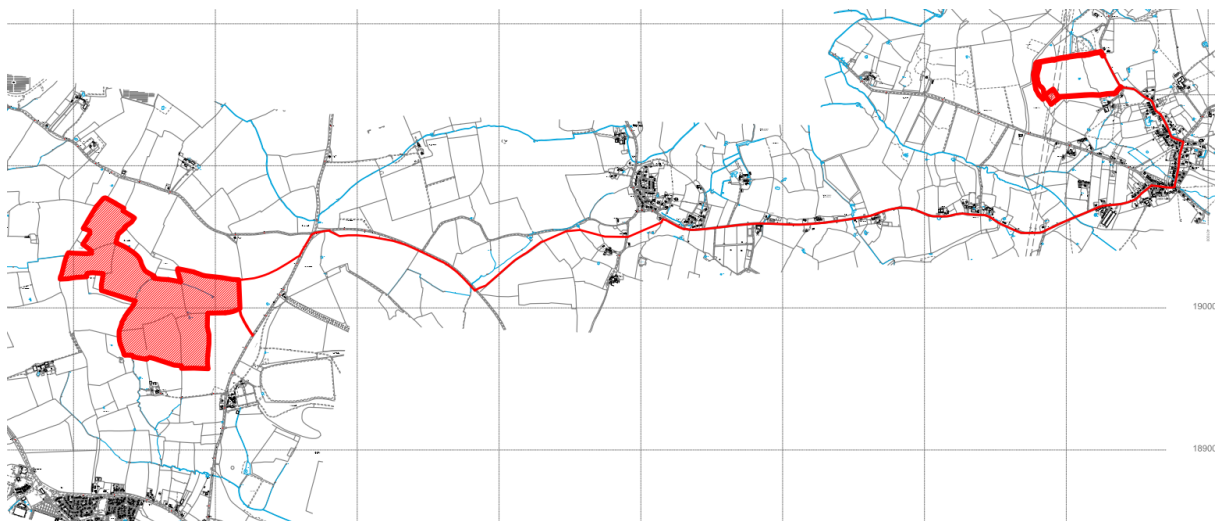
Route of underground cable connection between proposed Solar Farm Site and DNO compound – site outlined in red
